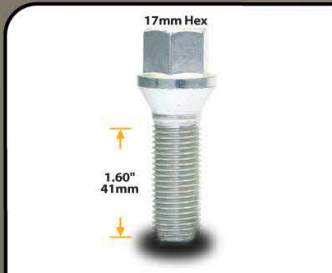
17mm Hex Lug Bolt - Cone Seat PART # 075160 THREAD SIZE 12mm x 1.50 x 1.60"
