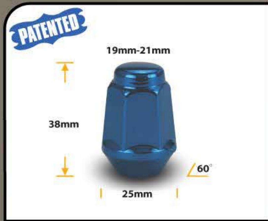
Duplex Taper Lug Nut - Blue PART # THREAD SIZE 811838BL 3/8"-24 811840BL 7/16"-20 811842BL 1/2"-20 811844BL 12mm x 1.25 811845BL 12mm x 1.50 811850BL 12mm x 1.75 811848BL 14mm x 1.50 811873BL 14mm x 2.00
