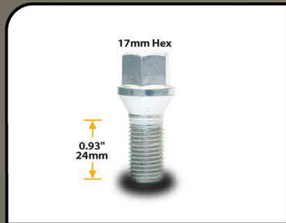
17mm Hex Lug Bolt - Cone Seat PART # 075093 THREAD SIZE 12mm x 1.50 x 0.93"
