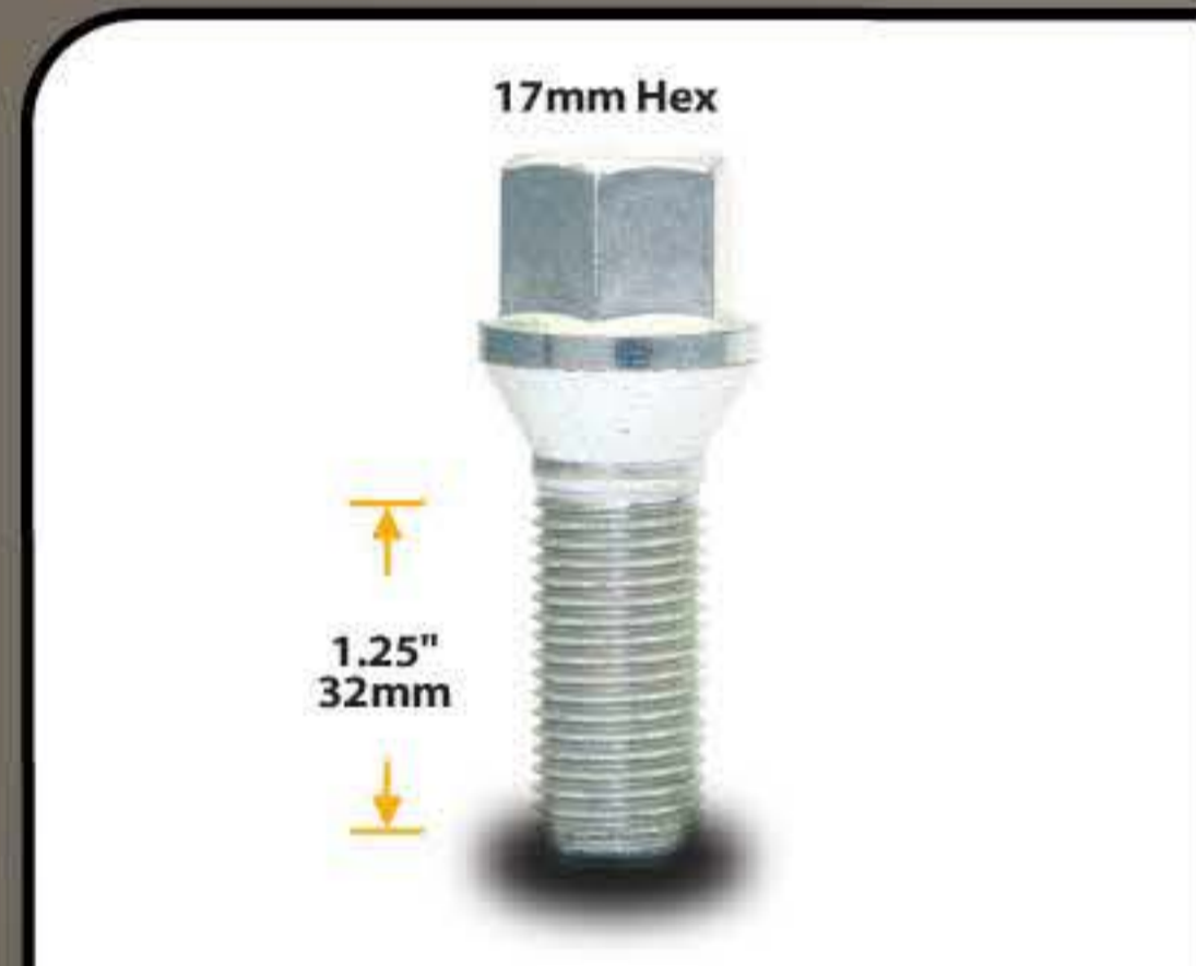
17mm Hex Lug Bolt - Cone Seat PART # 074125 THREAD SIZE 14mm x 1.50 x 1.25"
