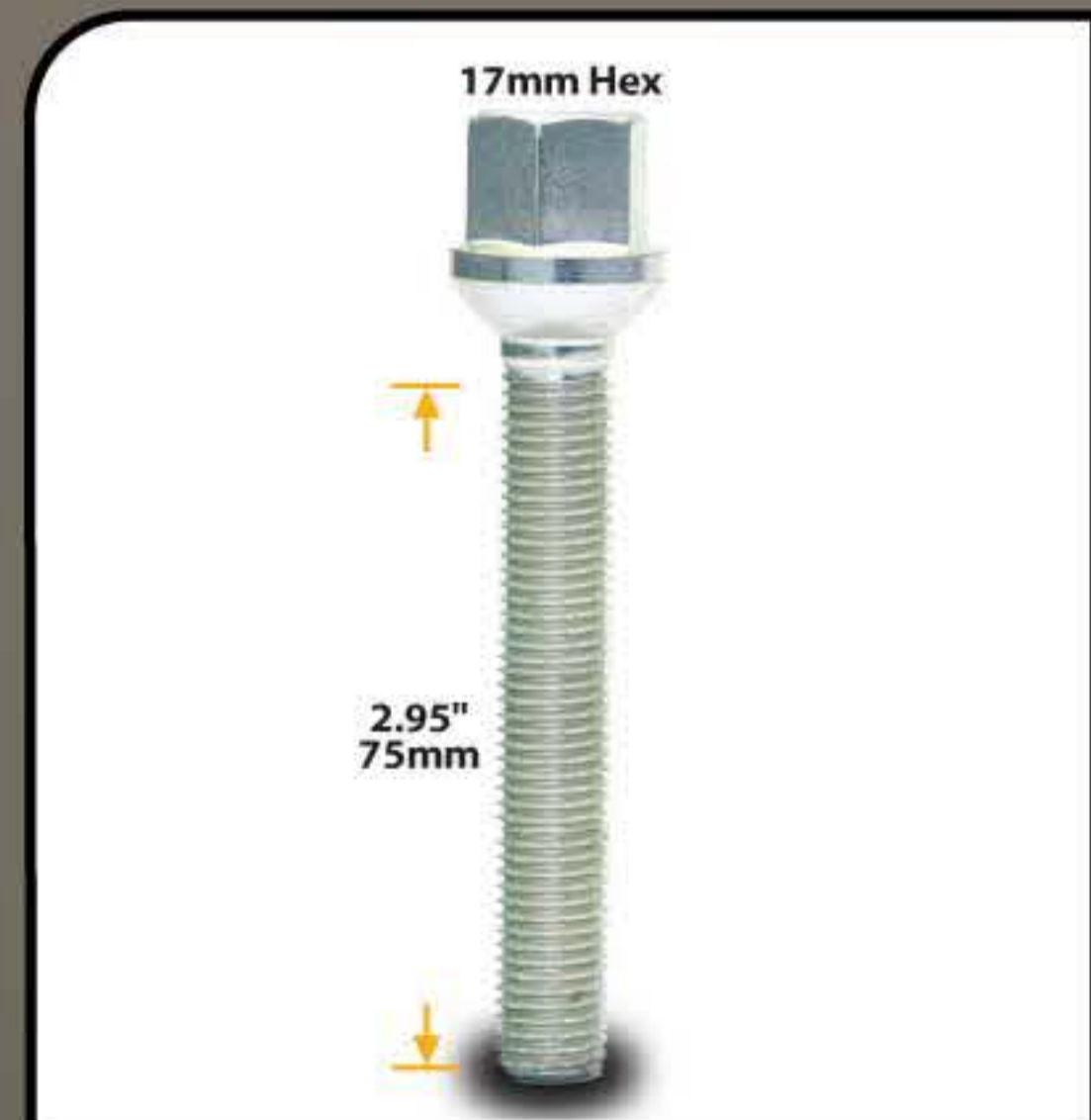
17mm Hex Lug Bolt - Ball Seat PART # 085295, 084295 THREAD SIZE 12mm x 1.50 x 2.95", 14mm x 1.50 x 2.95"
