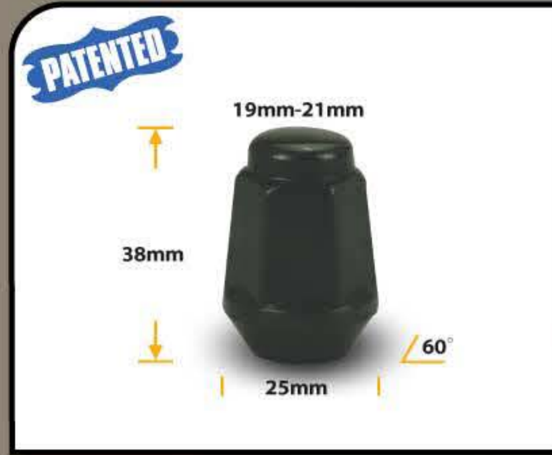
Duplex Taper Lug Nut - Black PART # THREAD SIZE 811838BC 3/8"-24 811840BC 7/16"-20 811842BC 1/2"-20 811844BC 12mm x 1.25 811845BC 12mm x 1.50 811850BC 12mm x 1.75 811848BC 14mm x 1.50 811873BC 14mm x 2.00
