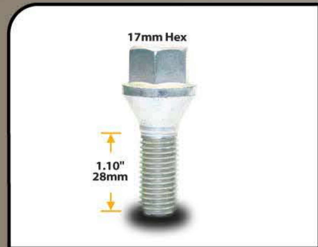
17mm Hex Lug Bolt - Cone Seat PART # 075110 THREAD SIZE 12mm x 1.50 x 1.10"
