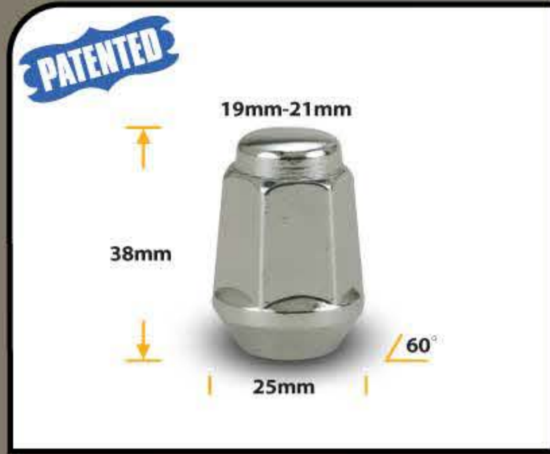
Duplex Taper Lug Nut PART # THREAD SIZE 811838 3/8"-24 811840 7/16"-20 811842 1/2"-20 811844 12mm x 1.25 811845 12mm x 1.50 811850 12mm x 1.75 811848 14mm x 1.50 811873 14mm x 2.00
