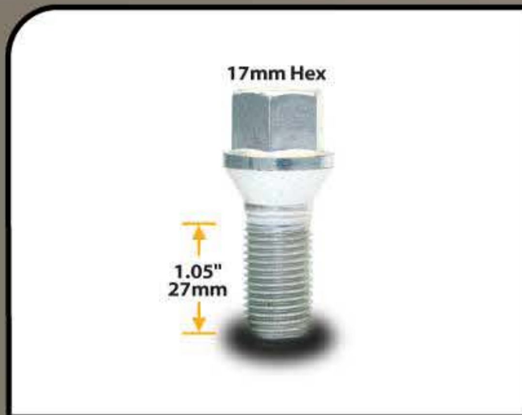
17mm Hex Lug Bolt - Cone Seat PART # 074105 THREAD SIZE 14mm x 1.50 x 1.05"
