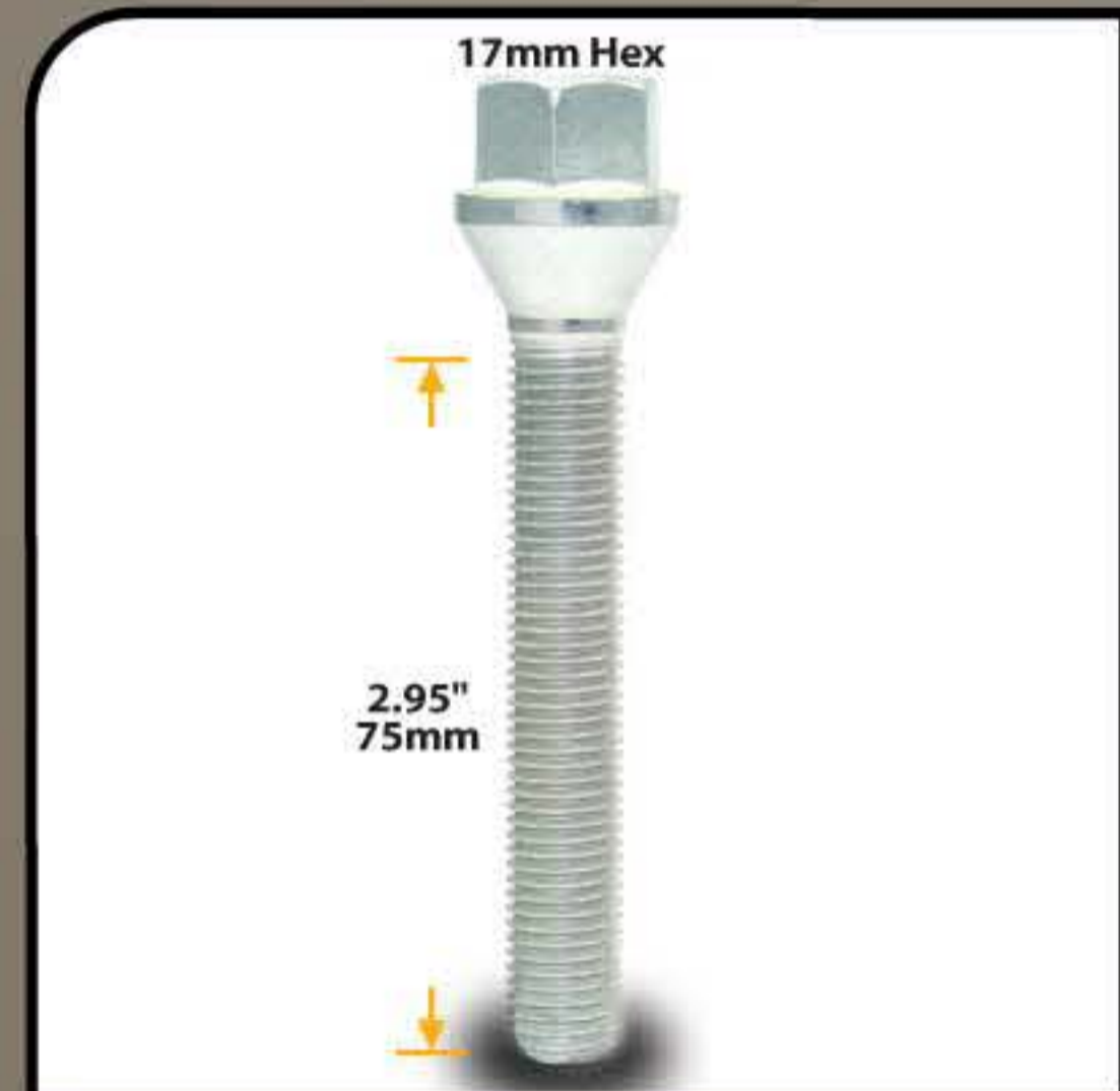
17mm Hex Lug Bolt - Cone Seat PART # 072295, 075295, 074295 THREAD SIZE 12mm x 1.25 x 2.95", 12mm x 1.50 x 2.95", 14mm x 1.50 x 2.95"
