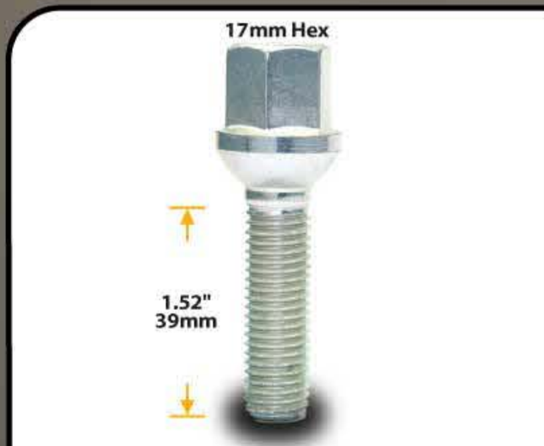
17mm Hex Lug Bolt - Ball Seat PART # 085152 THREAD SIZE 12mm x 1.50 x 1.52"
