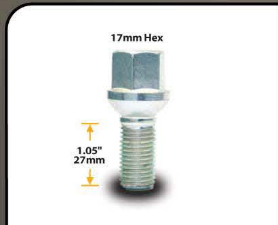
17mm Hex Lug Bolt - Ball Seat PART # 084105 THREAD SIZE 14mm x 1.50 x 1.05"
